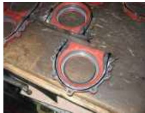
Application of flange sealant on engine flywheel housing seal cover
