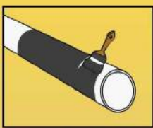
Priming pipes, rods and cables.
